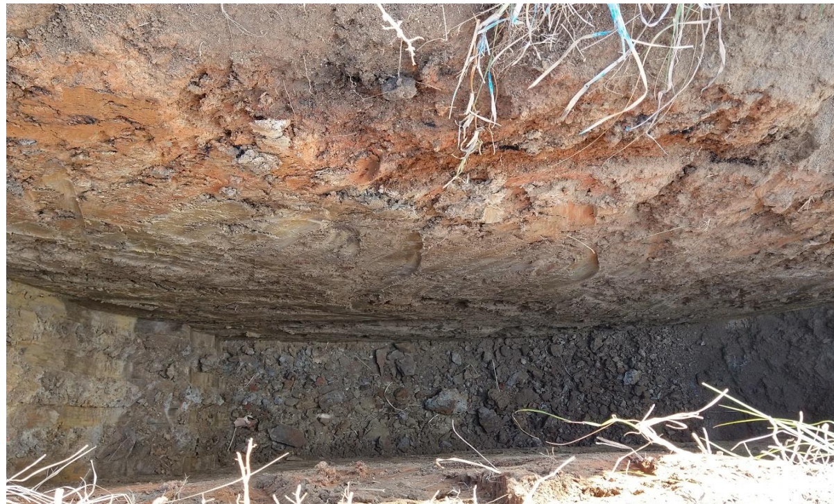
Photo 7: Test Pit 117 profile (Refusal at 2.2m) Typical of central and southern parts of Stage 2
