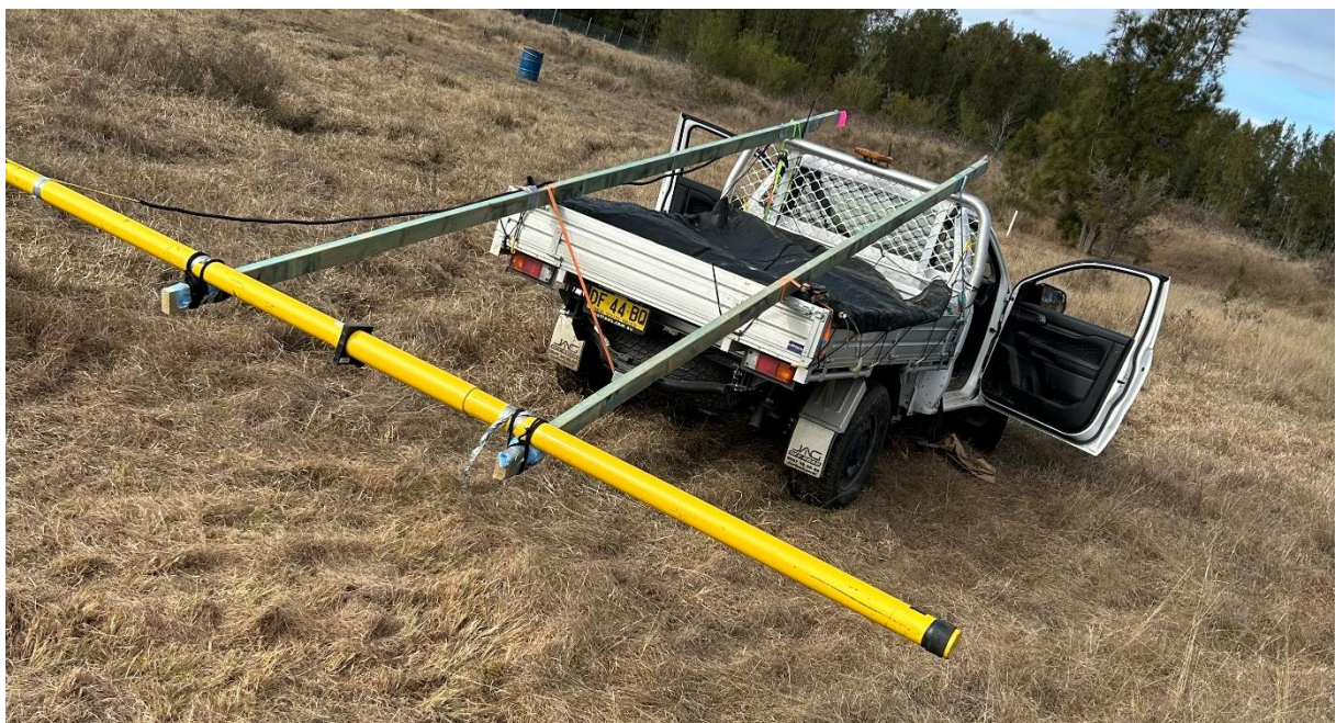
Figure 4: Dualem 42s extended behind 4WD vehicle.
