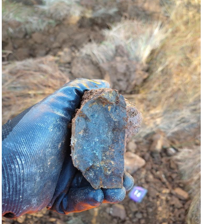
Photo 10: Basaltic material from base of Test Pit 123 - high strength
